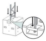
Scaffold tubes can be placed directly into the vertical tube inserts (x2) instantly providing a secure base for aluminium beam structures, for example height barrier or lighting truss rig.
