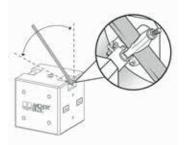
Scaffold tubes can be attach direct via a right-handed coupler to the top scaffold tubes. These can be rotated through a variety of angles to brace other scaffolding or fencing as shown above.
